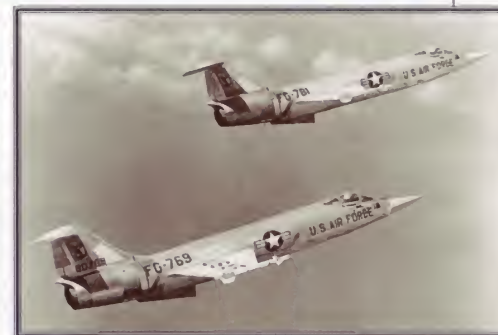
▶ Wingtip missiles Originally designed for US Navy aircraft, the early versions of the Sidewinder missile were brought into USAF service with the F-104. They initially proved only marginally more reliable than the Starfighter.
